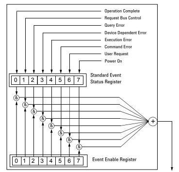
Figure 3-2 Standard Event Status Register Diagram
