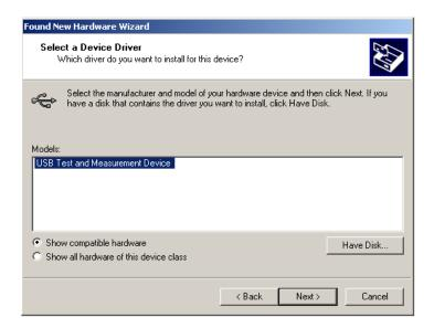
The wizard will guide you through the rest of installation till the driver is installed. Run Keysight IO libraries suite, the analyzer will be detected automatically.
