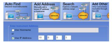
6 Press "Test Connection" to check the LAN connection. The figure below indicates that the connection is ready.
