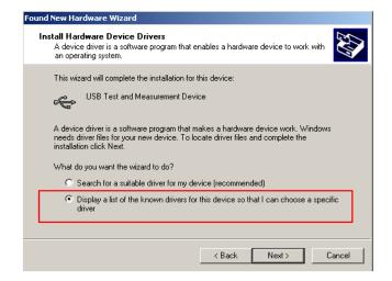
7 PC will detect the instrument automatically. The item "USB Test and Measurement Device" displays in the pop-up window. Select it and press Next.
